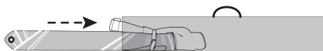
Fig. 11: Insert with the sleeve-end first into the sail bag and store horizontal.
