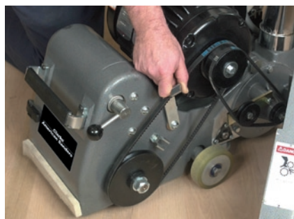
The quick release drive belt tension system eases disassembly and storage.
