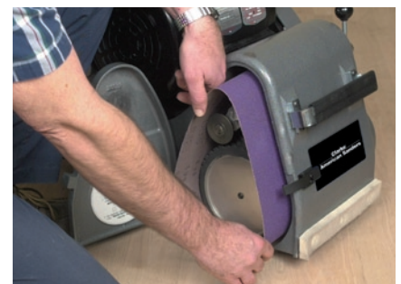
The recessed drum door provides better air seal and eases abrasive installation and adjustments.
