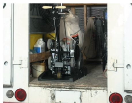
A unique transport platform bolts into vehicles for easy storage and transport.
