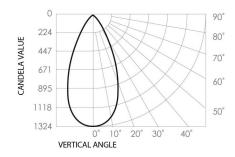
Lumen output: 780lm Colour temp.: 3000K Efficacy: 65lm/W Beam angle: 55°
